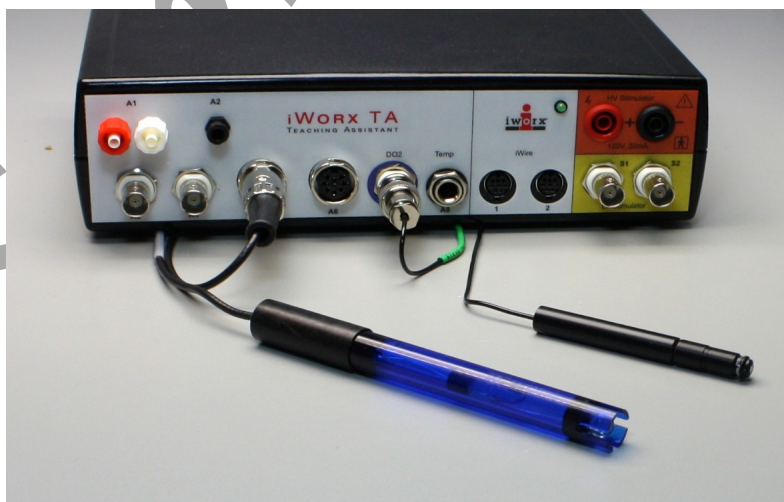
Figure GB-4-S4: The ISE-730 dissolved oxygen probe and pH probe connected to the IXTA.
