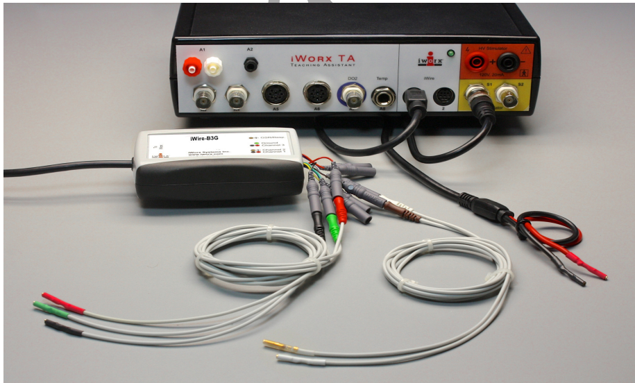
Figure AN-4-S1: The iWire-B3G recording cable and C-BNC-P2 stimulator cables attached to the IXTA.
