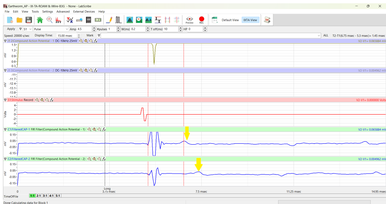
Figure AN-4-L5: The monophasic action potential shown on both channel 1 and channel 2 of the earthworm action potential recording for the long path setup.
