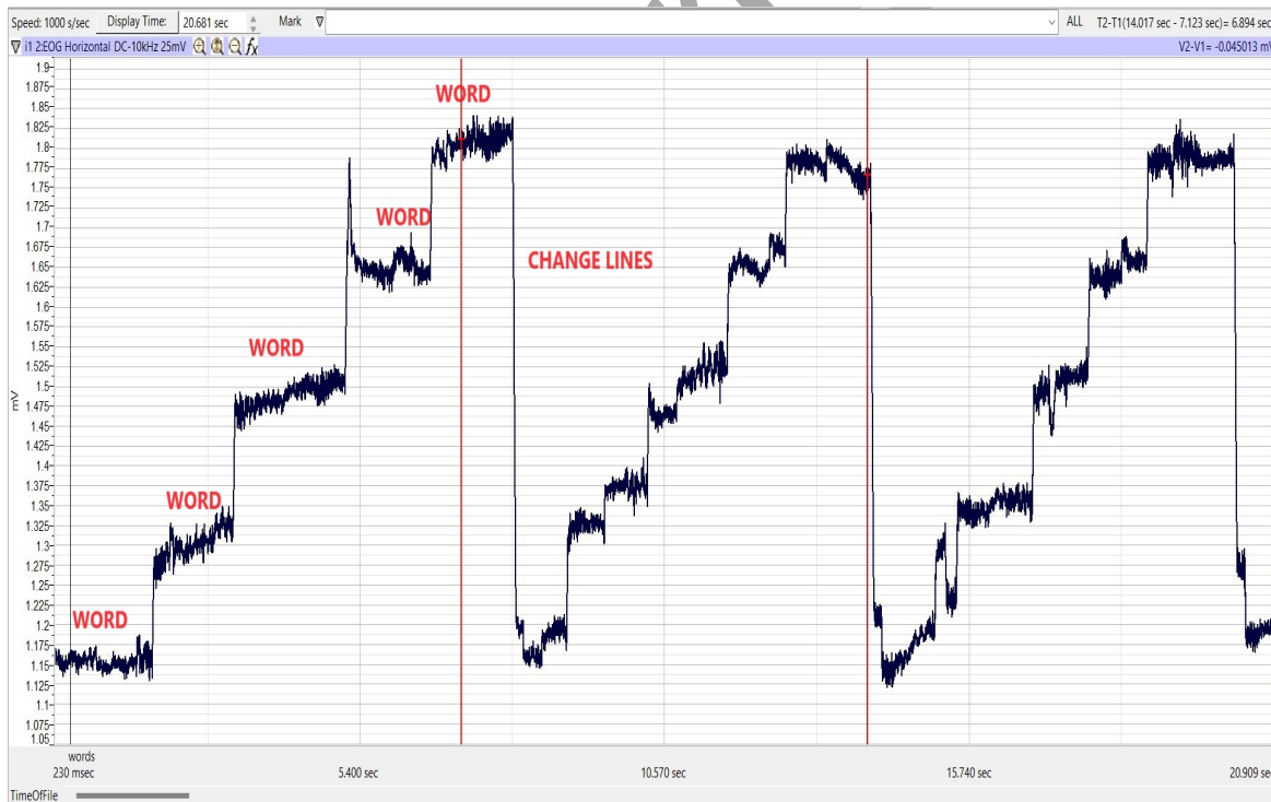
Figure HM-3-L1: Electroculogram (EOG) of a subject reading slowly. Four words are on each line. As the subject moves his eyes to the right to read the next word, the level of the recording rises a step. As the subject moves his eyes back to the beginning of the next line, the amplitude of the EOG drops.
