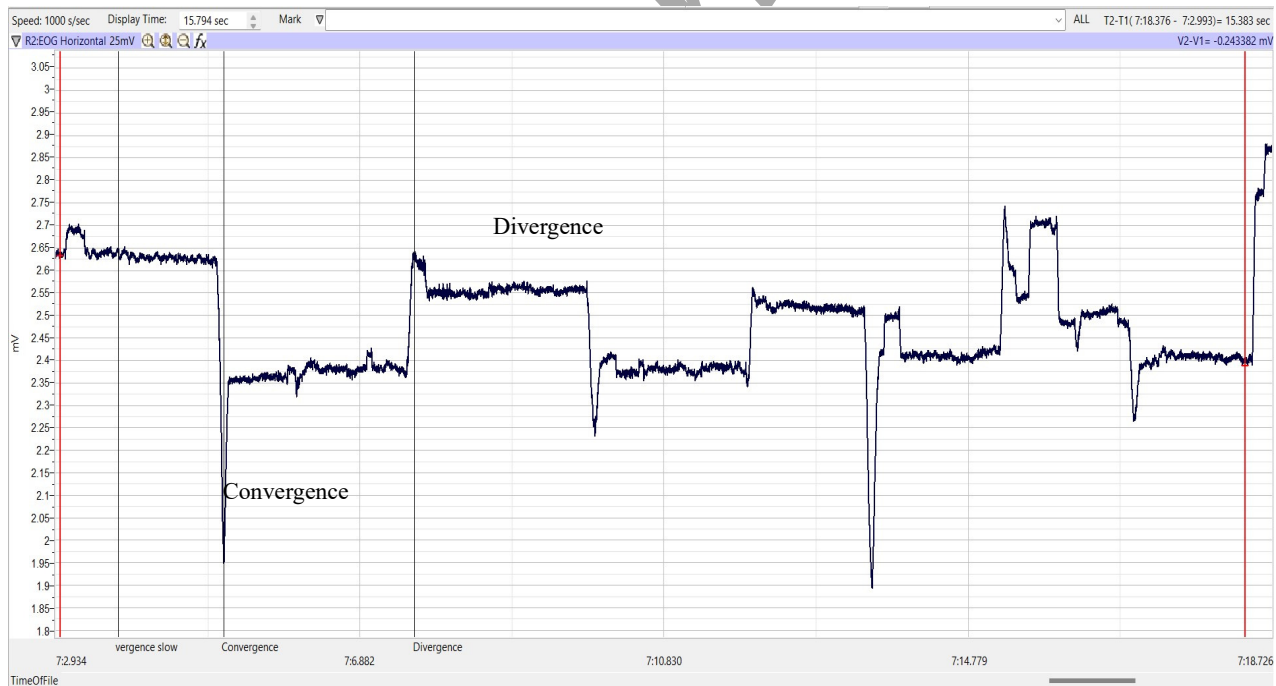
Figure HM-3-L4: Electroculogram (EOG) of a subject focusing on distant and near targets. Note – the trace may be inverted depending on electrode placement.
