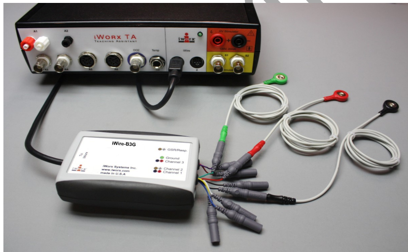
Figure HM-3-S1: The EOG cable connected to an IXTA.
