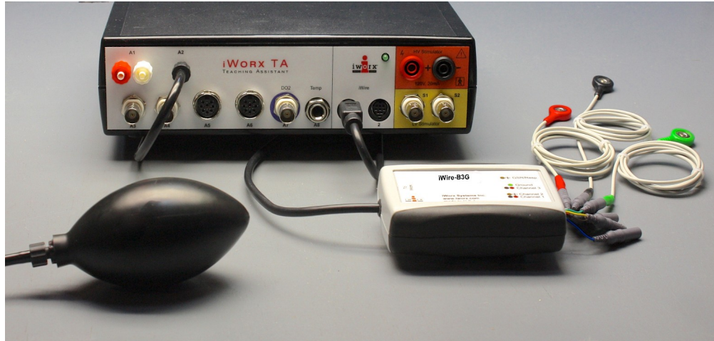
Figure HM-1-S2: The EMG cable and hand dynamometer connected to an IXTA.
