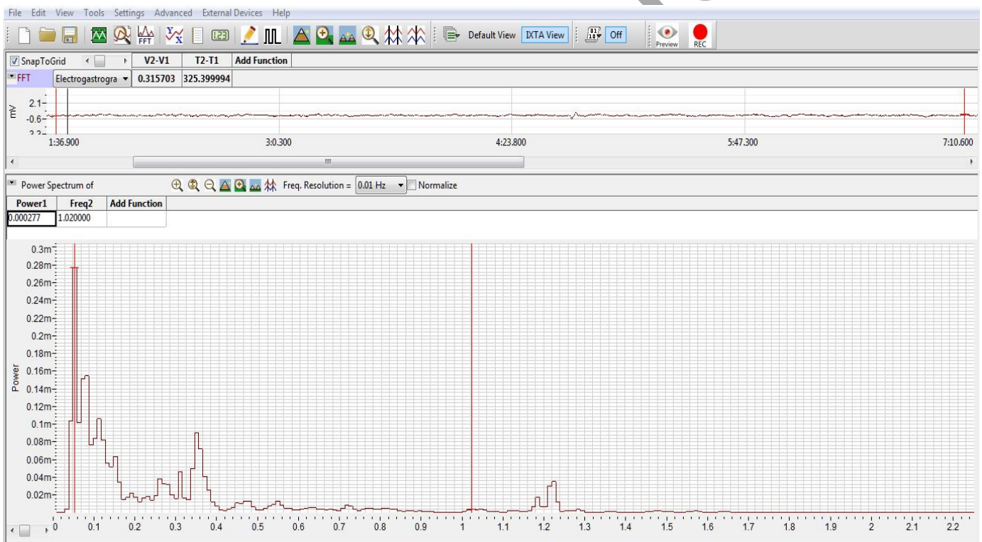
Figure HM-8-L4: The frequency and power of the EGG shown in the FFT window. The left hand cursor is placed on the peak of the highest wave in the histogram. The frequency and power are shown in the upper left of the graph.
