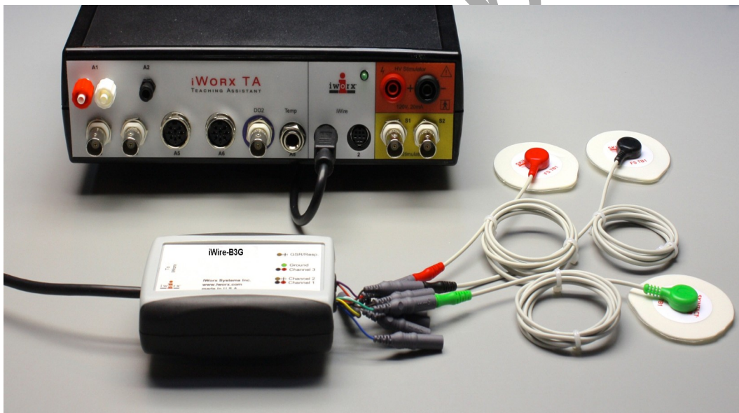
Figure HM-8-S1: The iWire-B3G EGG cable and leads connected to an IXTA.
