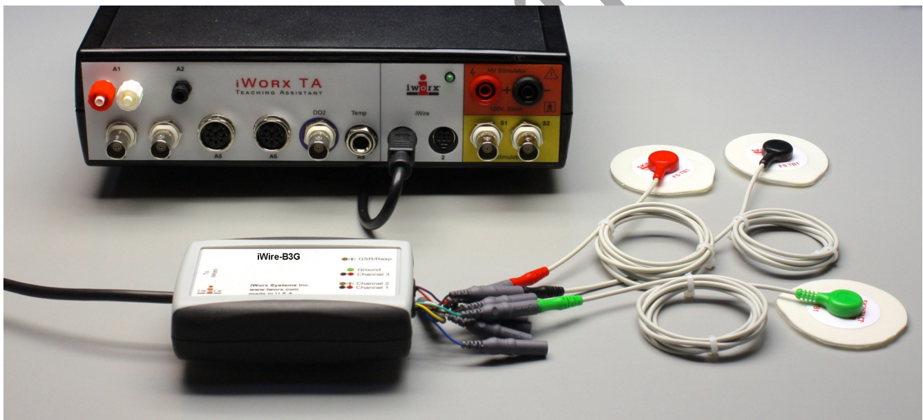
Figure HC-6-S1: The iWire-B3G ECG cable with three lead wires attached.
