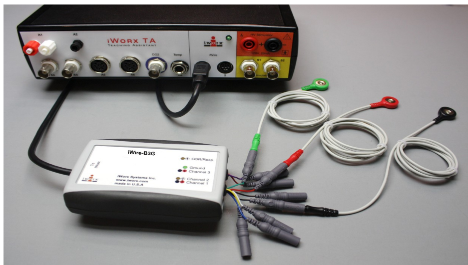
Figure HH-11-S1: The iWire-B3G ECG cable with three lead wires attached connected to the IXTA.
