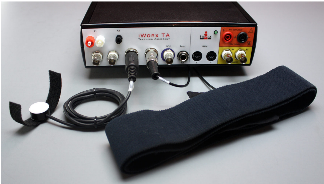
Figure HH-5-L6: The RM-204 connected to the IXTA.
