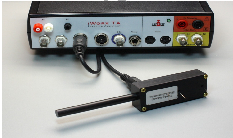
Figure AM-7-S2: The FT-302 force transducer connected to the IXTA.
