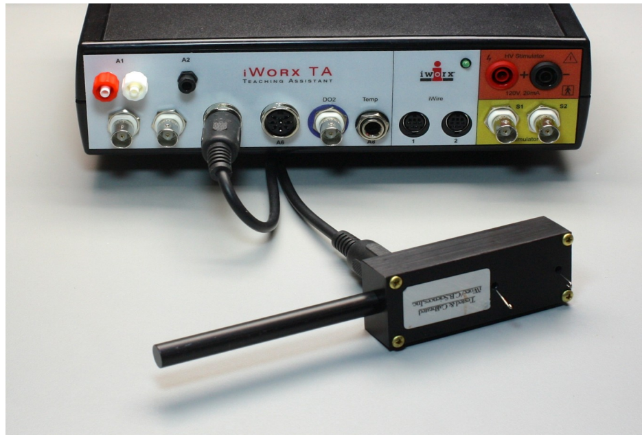
Figure AM-9-S2: The FT-302 force transducer connected to the IXTA.
