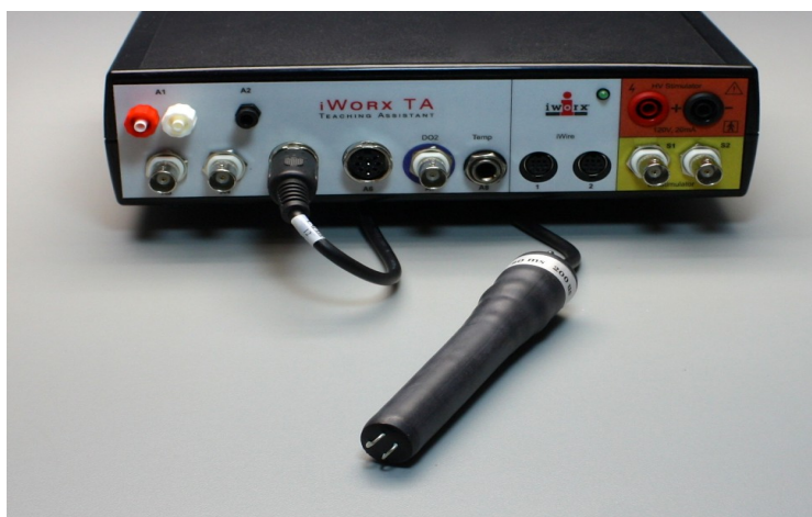
Figure GB-6-S2: The CM-100 conductivity meter connected to the IXTA.
