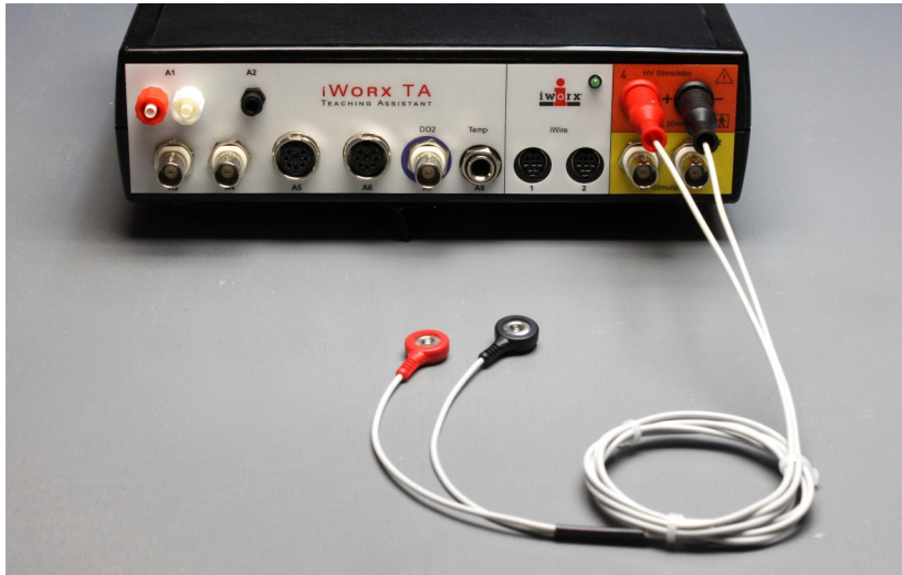
Figure HN-13-S3 and HN-13-S4: HV stimulator cables connected to the IXTA and connected to the hand. The black electrode is on the outside of the hand, the red electrode on the back of the hand.
