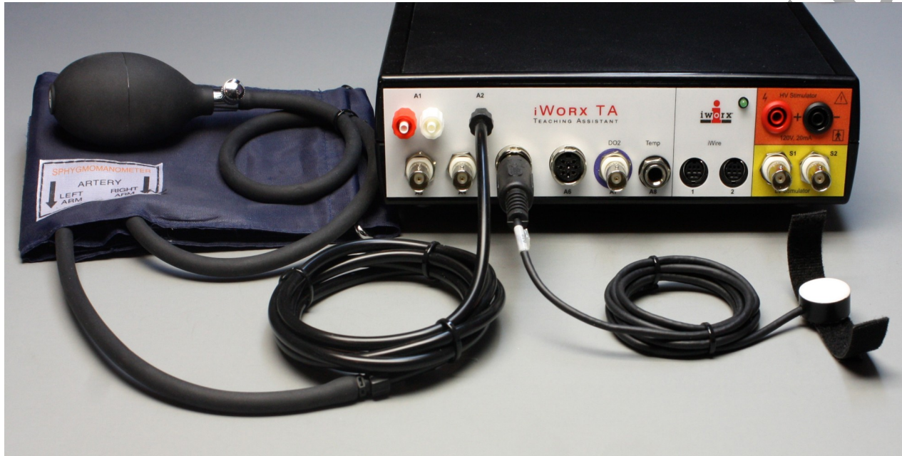
Figure HC-5-S3: The PT-104 pulse transducer and the BP-220 non-invasive blood pressure transducer connected to an IXTA.
