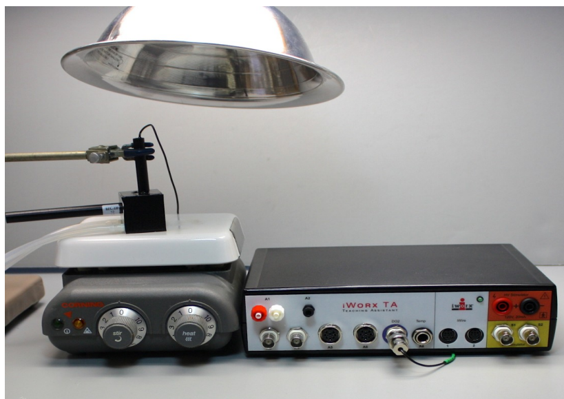
Figure CM-5-S4: The oxygen polarograph used to record photosynthetic electron transport. Black tape should cover the side of the polarograph block facing the light source, except on the area directly on the front of the chamber. The light is focused on this open area so that the circle of light is only large enough to cover the chamber.
