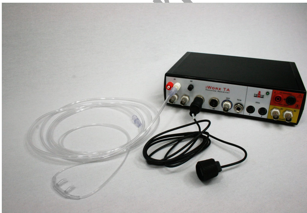
Figure HS-5-S3: The PT-104 and RM-220 connected to an IXTA.
