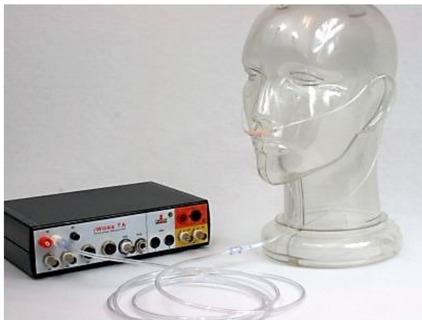
Figure HS-5-S2: The RM-220 nasal cannula attached to the IX-TA and showing the correct position on the head.
