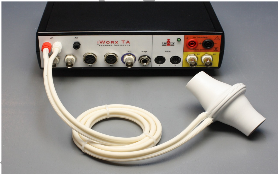
Figure HS-1-S2: The flowhead connected to the internal spirometer of the IXTA unit.
