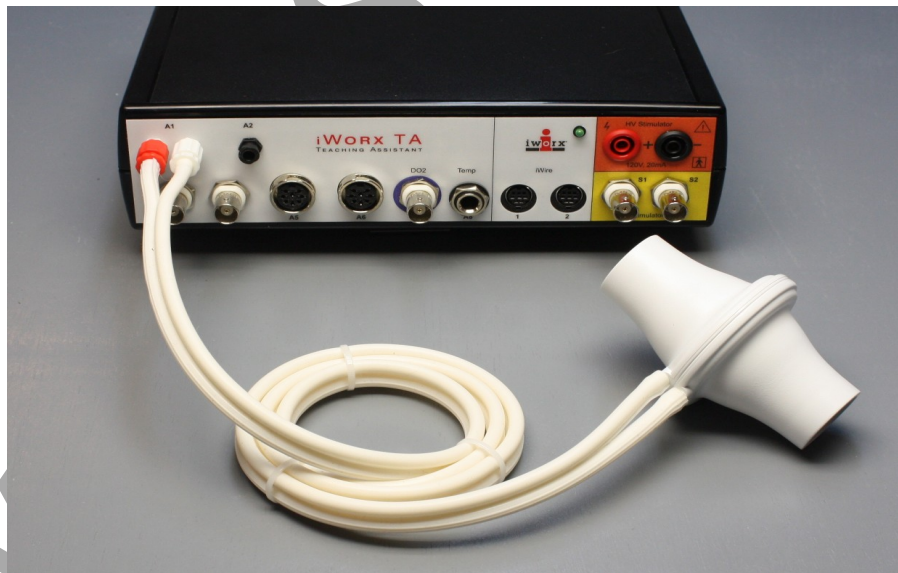
Figure HS-3-S2: The flow head connected to the internal spirometer of the IXTA unit.
