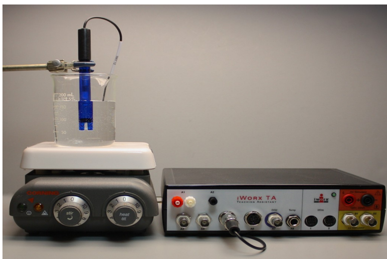
Figure GB-1-S2: The arrangement of the stirrer, pH electrode, and beaker for the calibration of the pH probe.
