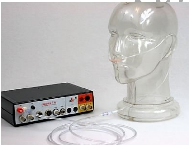
Figure HP-14-S3: Nasal cannula connected to the IX-TA and showing the proper positioning on the face.
