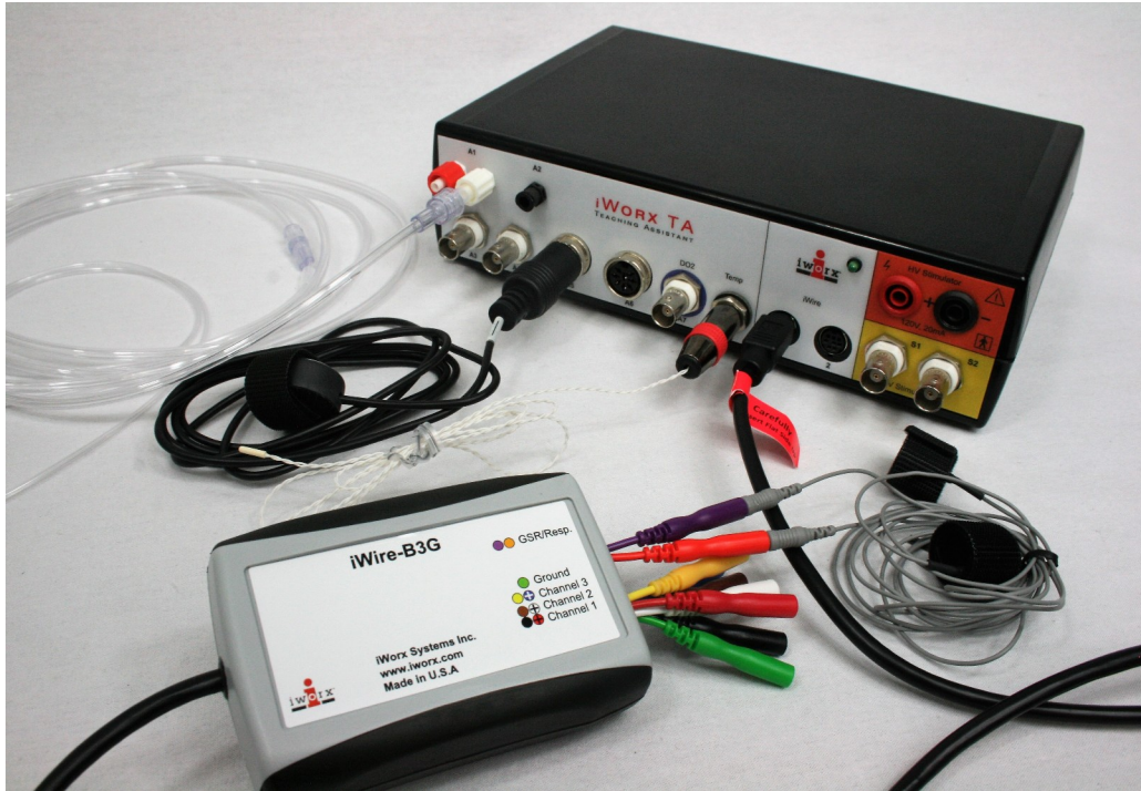
Figure HP-14-S4: The PT-104 pulse transducer, TM-220 temperature probe, GSR electrodes and the RM-220 nasal cannula connected to an IXTA.
