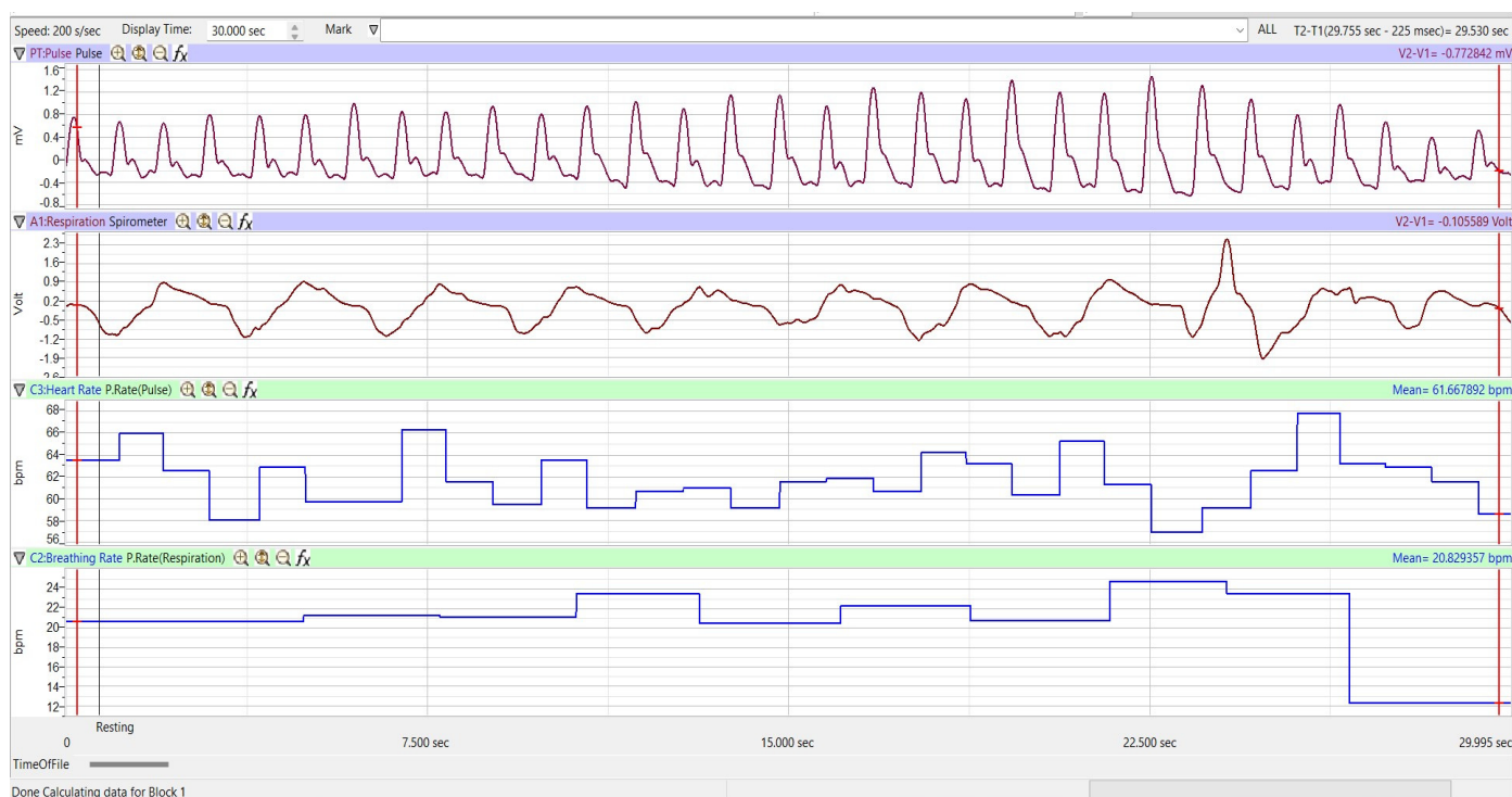
Figure HP-22-L2: Sample data showing pulse, heart rate, respiration and breathing rate.
