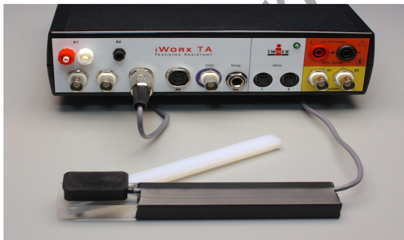
Figure HM-7-S2: A five lead EMG cable and Single-axis Goniometer connected to an IXTA.
