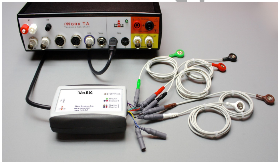
Figure HM-2-S1: A five lead EMG cable connected to an IXTA.
