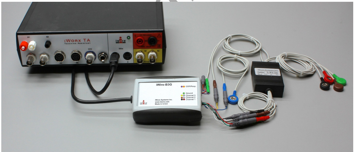
Figure HH-10-S1: iWire-B3G cable with the Wilson Terminal and the electrode cables attached to an IXTA for recording limb and chest lead ECG.
