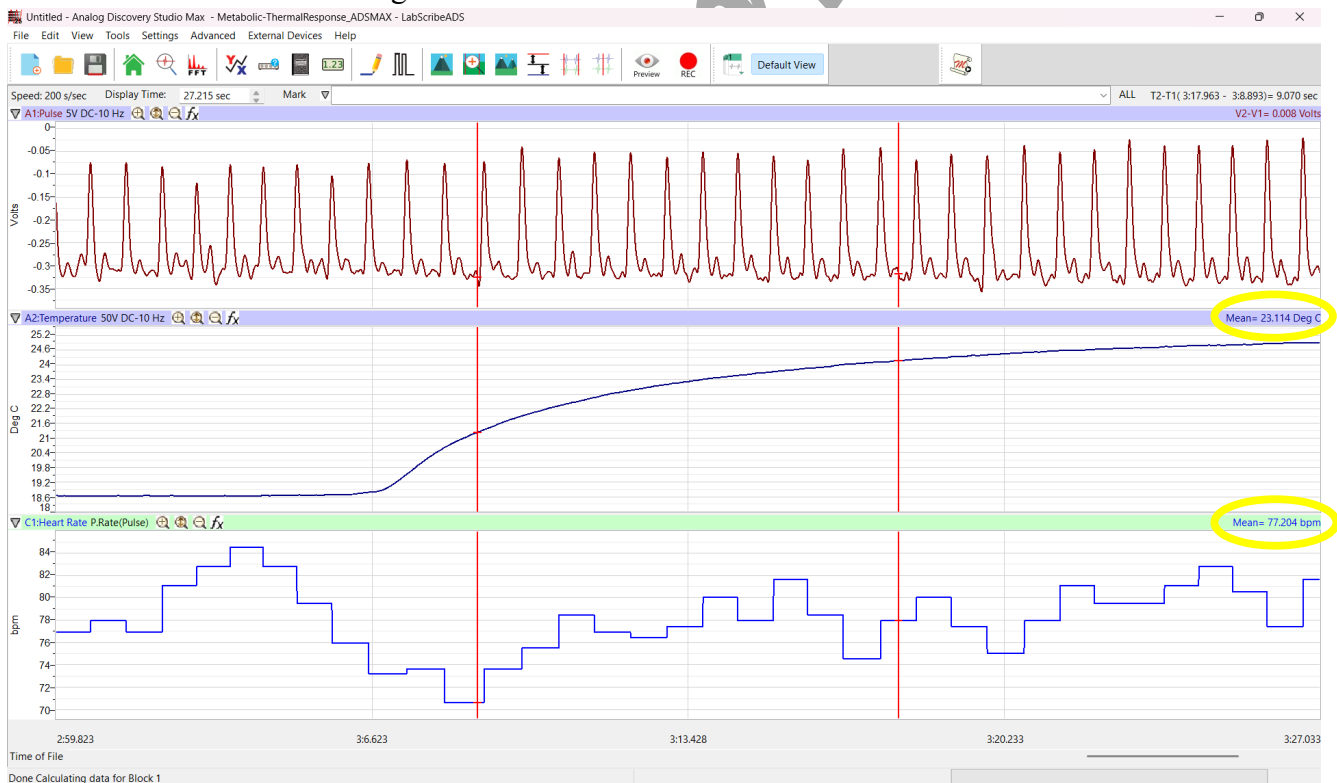
Figure ADS-BIA-2-L3: Polar heart rate monitor, skin temperature, and heart rate recordings while subject is at rest, showing the Mean values highlighted.
