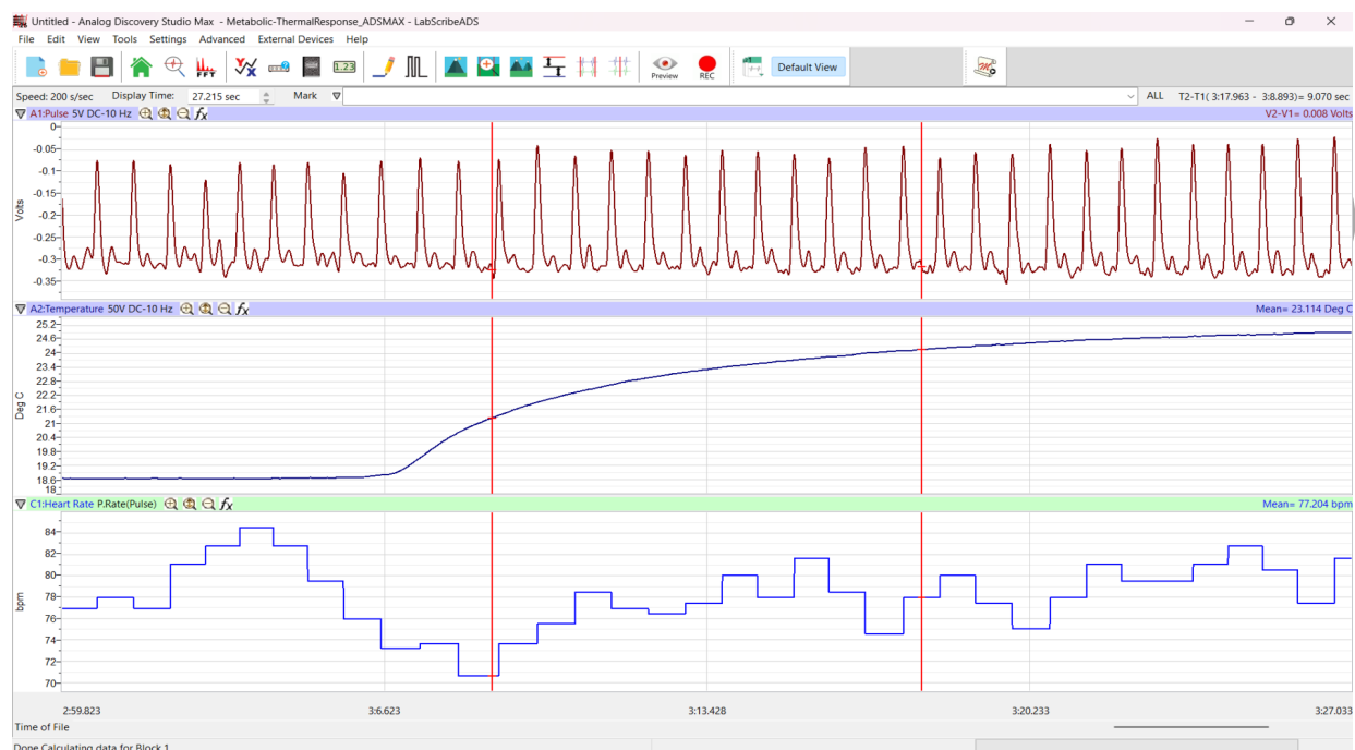
Figure ADS-BIA-2-L1: Pulse, skin temperature, and calculated heart rate recordings while subject is at rest, displayed in the Main window.
