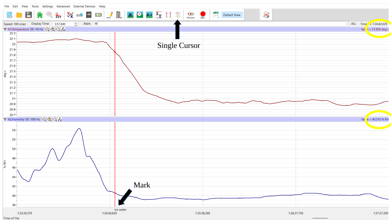
Figure ADS-CEK-3-S1: Recording of temperature and relative humidity after placing ice water beneath the sensors. A single cursor is positioned over the “Ice Water” mark to display the corresponding measurements on the right of each channel. The temperature reads 21.856 °C, and the relative humidity reads 40.5%.
