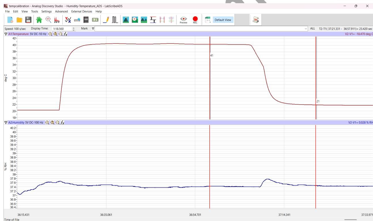
Figure ADS-CEK-3-S3: Temperature sensor calibration data. The sensor was calibrated with temperatures of 41 and 21 deg C.
