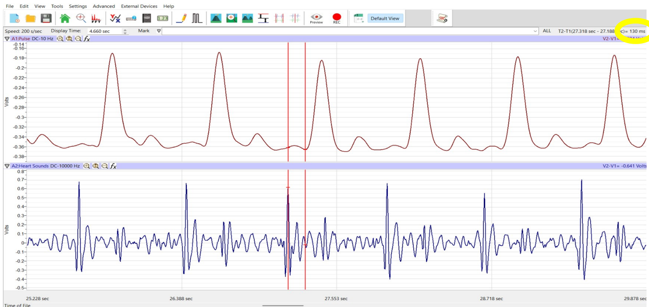
Figure ADS-BIA-5-L4: Recording of pulse and heart sounds displayed in the Main window. The pulse transit time (PTT), measured with the cursors, is 130 ms.
