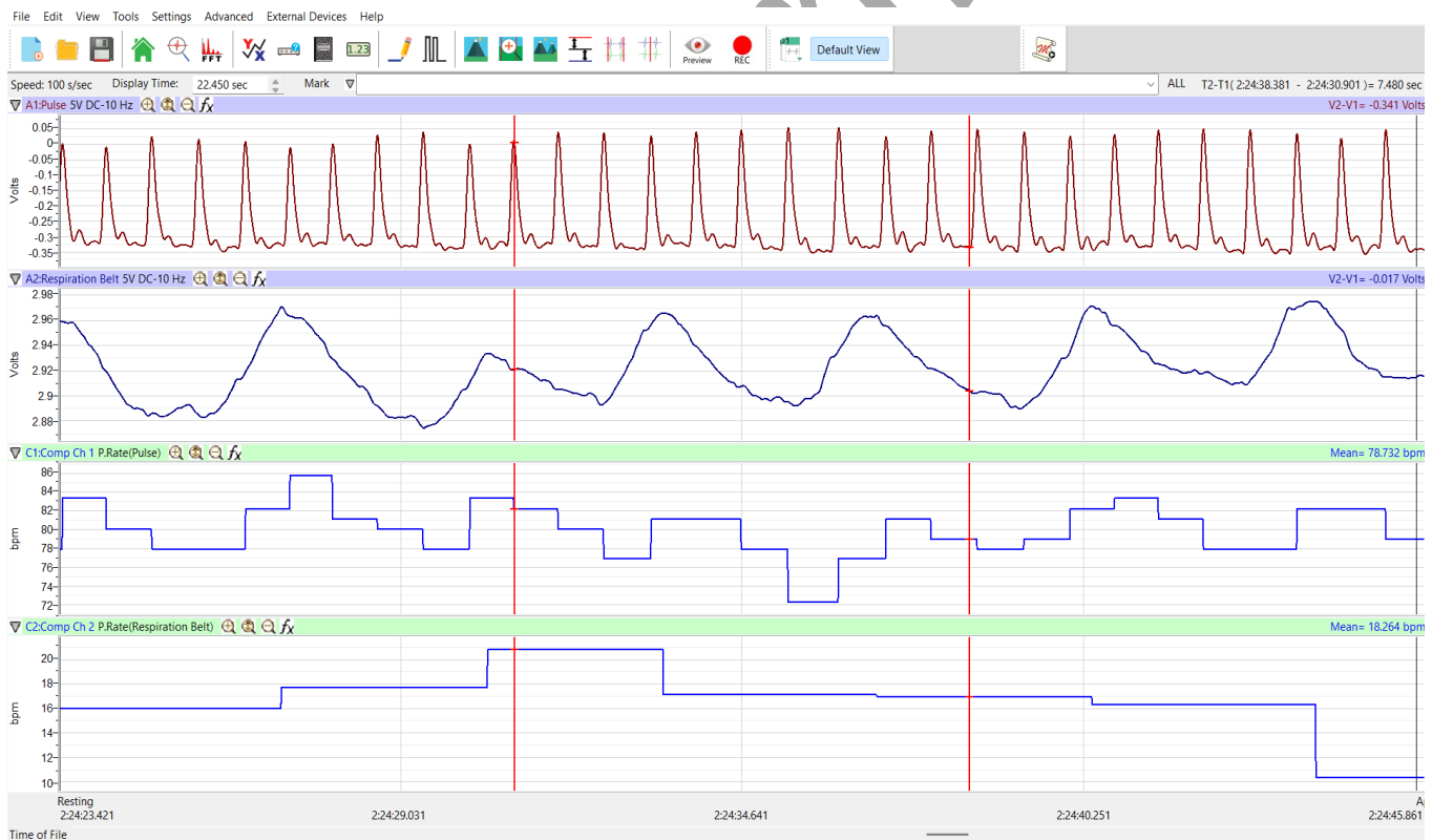
Figure ADS-BIA-1-L1: The pulse, respiration, heart rate, and breathing rate of a subject using abdominal breathing while at rest, displayed in the Main window.
