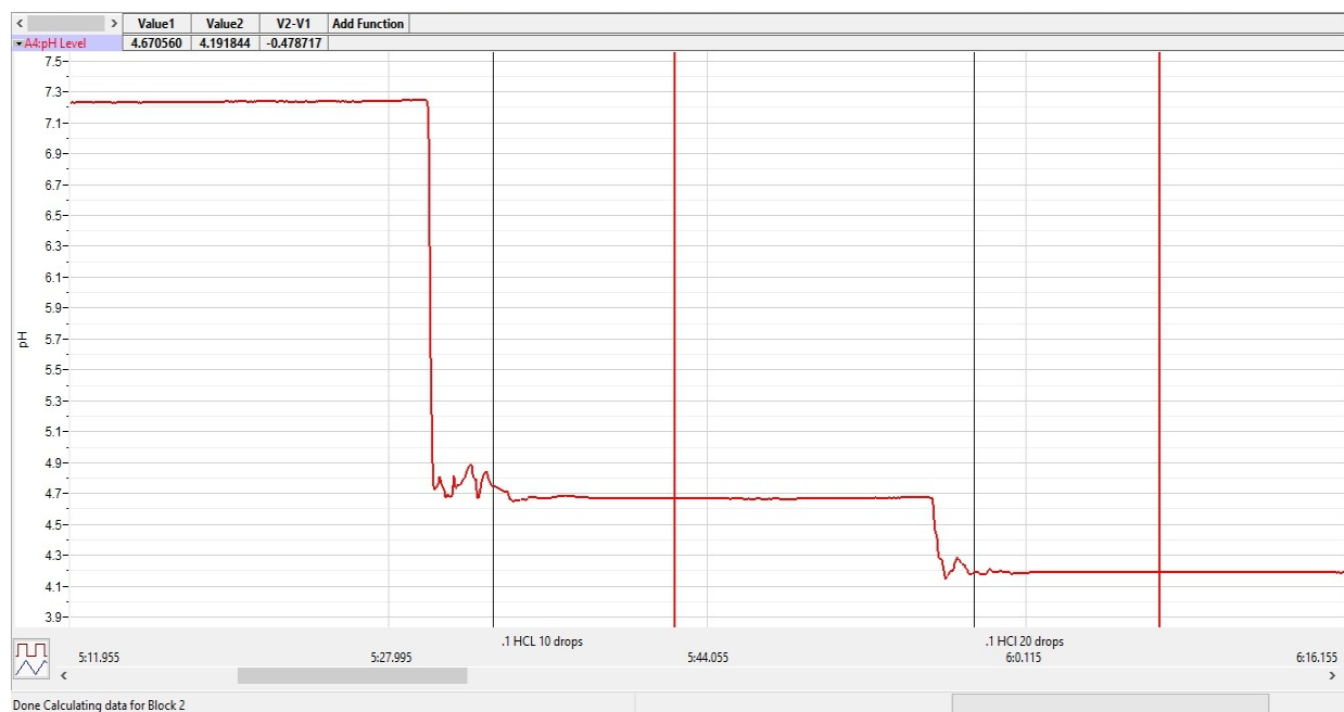
Figure ADS-CEK-4-L2: pH recording in the Analysis window showing the pH values for the addition of 0.1M HCl to the deionized water.
