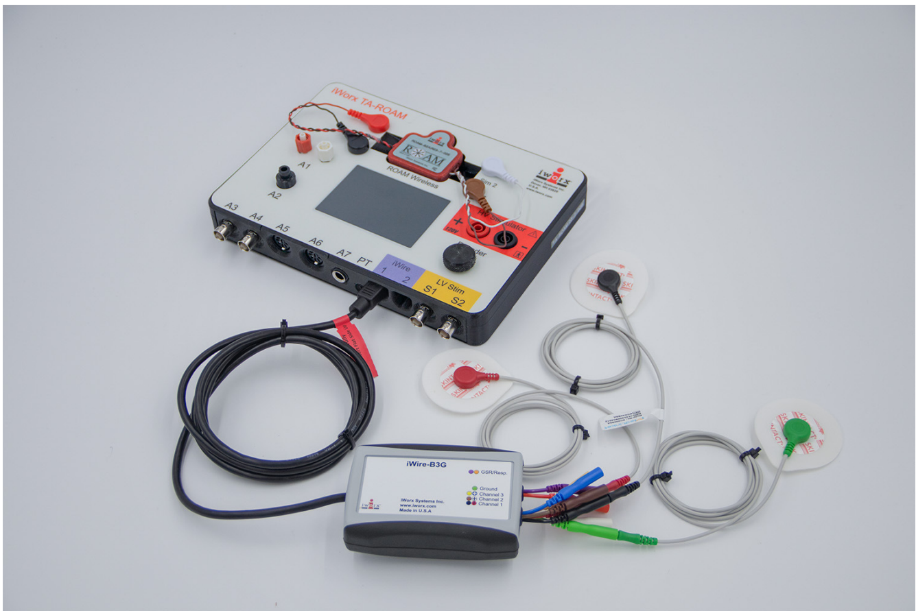
Figure HP-10-S1: The iWire-B3G cable connected to an IXTA.
