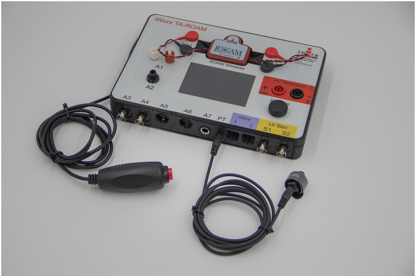
Figure HP-5-S2: The PPG-320 pulse transducer and the EM-220 event marker connected to an IXTA.
