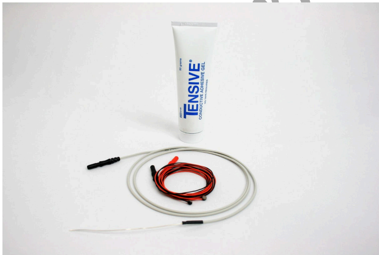
Figure GB-7-S1: The button & ground electrodes and tensive tac gel for this lab.
