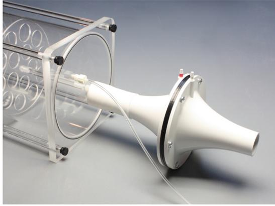
Figure HE-4-S15: 1000L flow head connected to the mixing chamber, showing the Nafion tubing connected to the outlet sampling port near the flow head.
