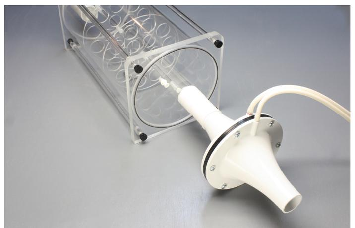
Figure HE-4-S2 and HE-4-S3: The mixing chamber showing the 1000L/min flow head connected to the outlet.
