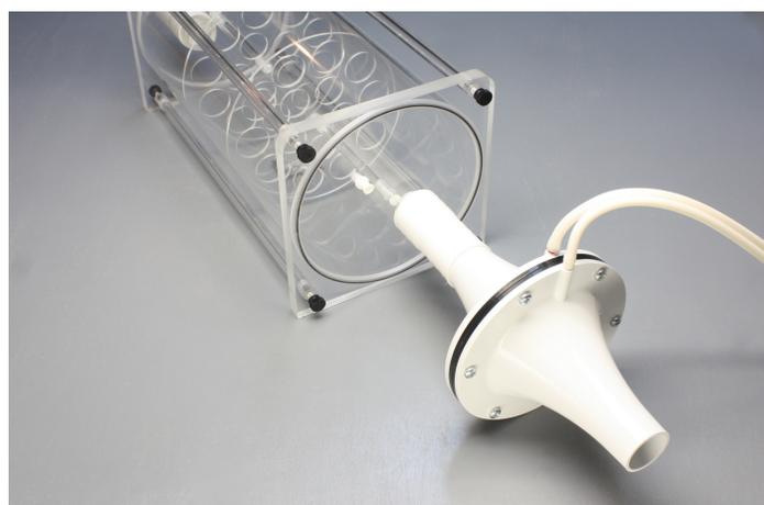
Figure HE-4-S2 and HE-4-S3: The mixing chamber showing the 1000L/min flow head connected to the outlet.
