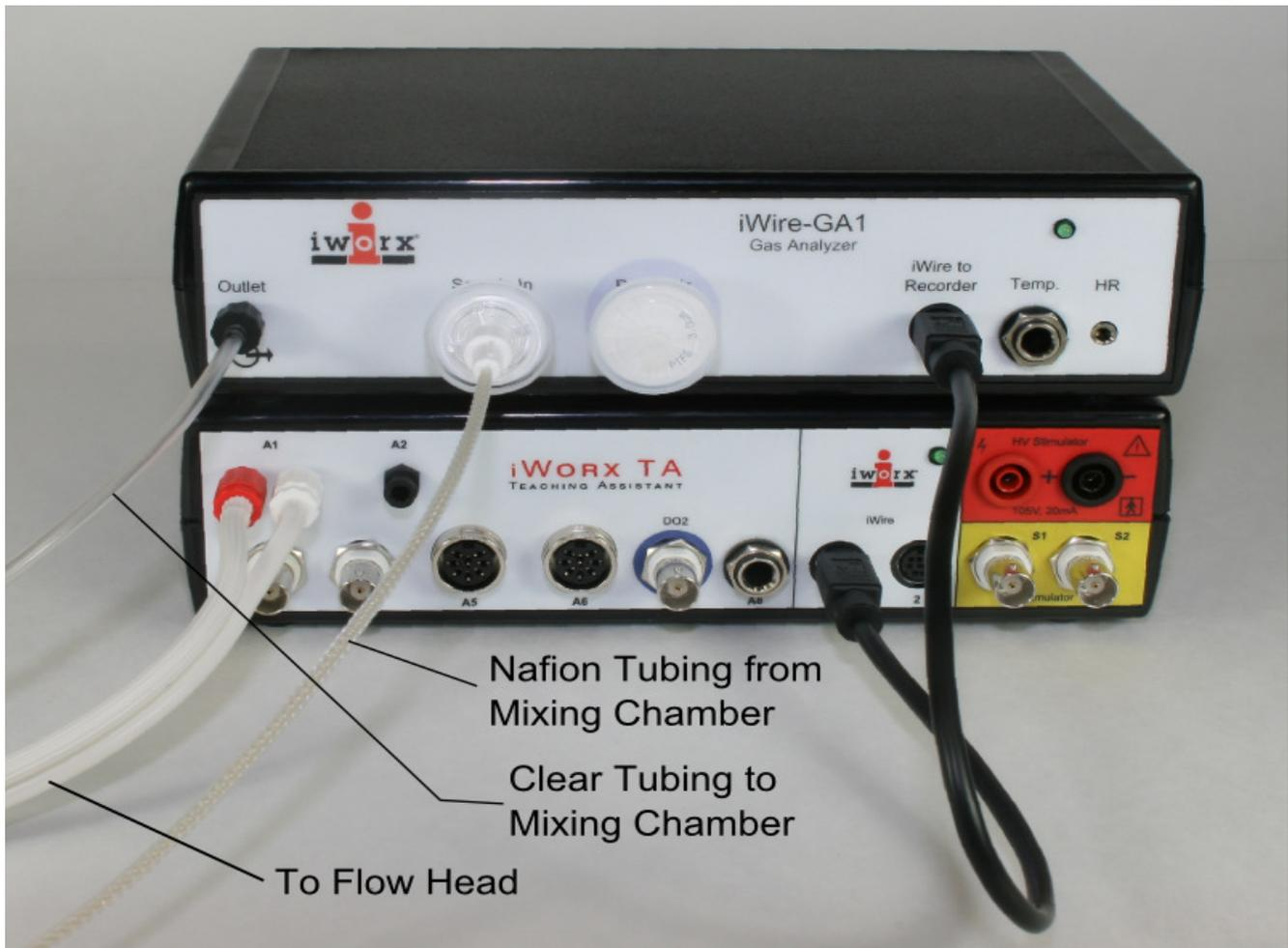
Figure HE-4-S4: The iWire-GA gas analyzer connected to an IXTA. All tubings are connect properly in this image.
