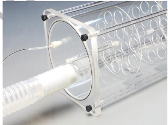
Figure HE-4-S16: 3 liter calibration syringe connected to the smooth bore tubing and Figure HE-4-S17: The smooth bore tubing connected to the mixing chamber.
