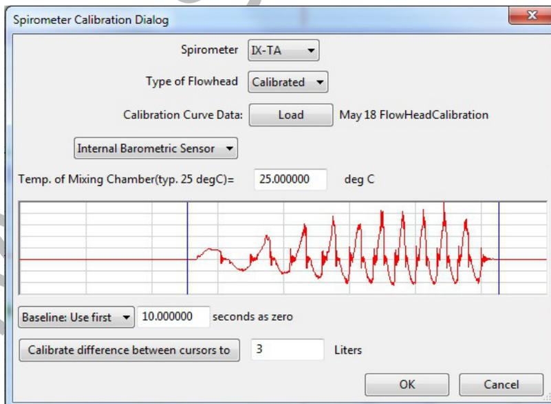
Figure HE-4-S10: Spirometer Calibration dialog window.
