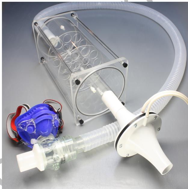
Figure HE-4-S6: The assembled devices used during metabolic studies. The assembly includes: the mixing chamber, smooth interior tubing, Nafion sampling tubing, flow head, spirometer, non-rebreathing valve, and mask.
