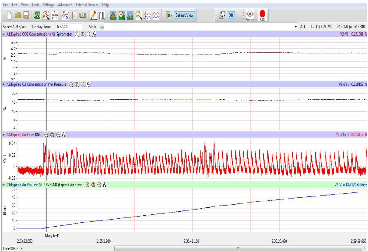
Figure HE-4-L2: Gas concentrations and volumes of a standing subject displayed on the Main window. Concentrations of gases reach a steady state after the mixing chamber is filled.
