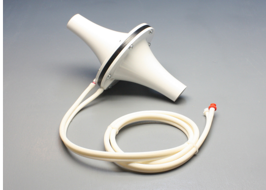
Figure HE-4-S1: The A-FH-1000 flowhead and the airflow tubing.
