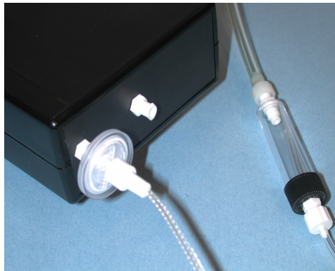
Figure HE-4-S10: A-CAL-150 attached to the rear of the GA-300 gas analyzer.
