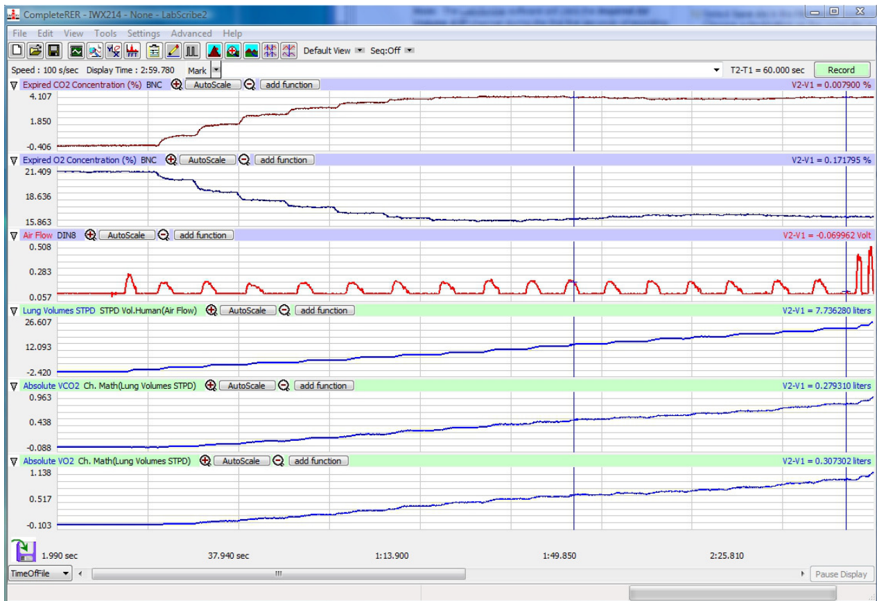
Figure HE-4-L1: Gas concentrations and volumes of a standing subject displayed on the Main window. Concentrations of gases reach a steady state after the mixing chamber is filled. Cursors placed one minute apart indicate VCO_2 is 0.302 liters and VO_2 is 0.337 liters. Therefore, RER is 0.90.
