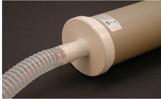
Figure HE-4-S17: 3 liter calibration syringe connected to the smooth bore tubing.
