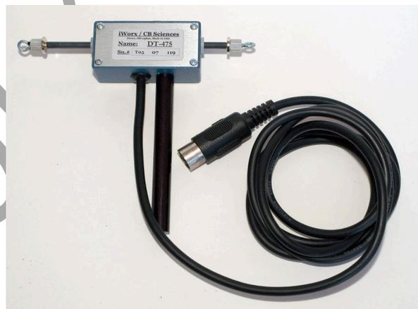
Figure AM-4-S1: The DT-475 displacement transducer.
