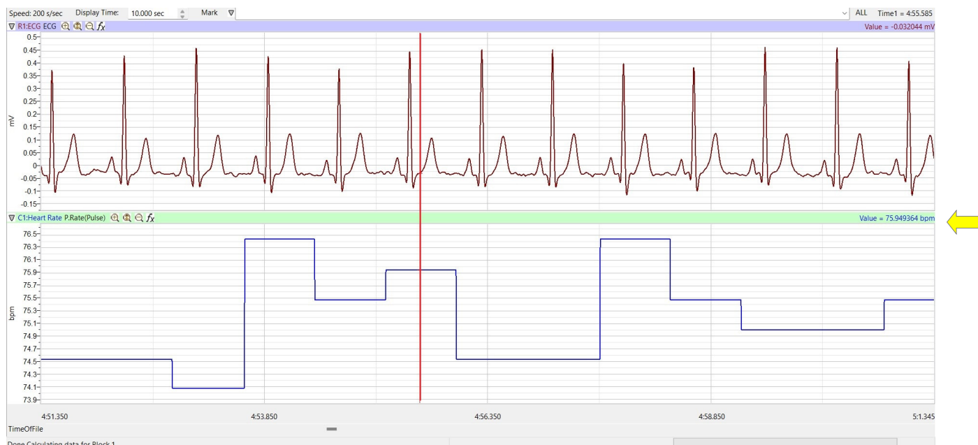
Figure T-T-L9: One cursor used to measure the heart rate of the subject from the data on the Heart Rate channel.
