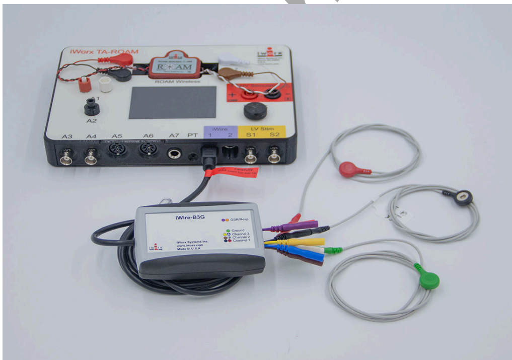
Figure T-T-S2: The iWire-B3G with three lead wires attached connected to the IX-TA.
