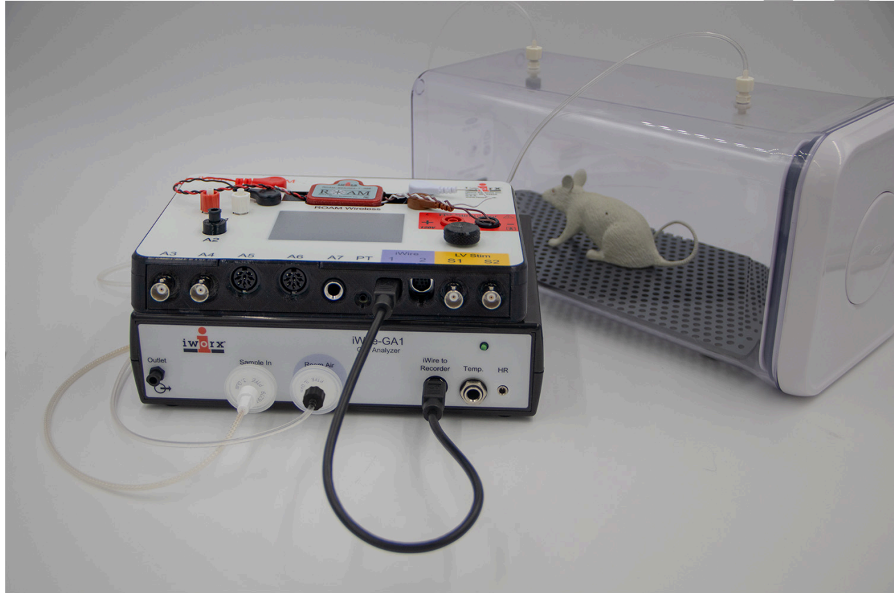
Figure AMe-1-S1: The front panel of both the IXTA and the iWire-GA showing the connections to and from the small animal chamber with the mouse inside.
