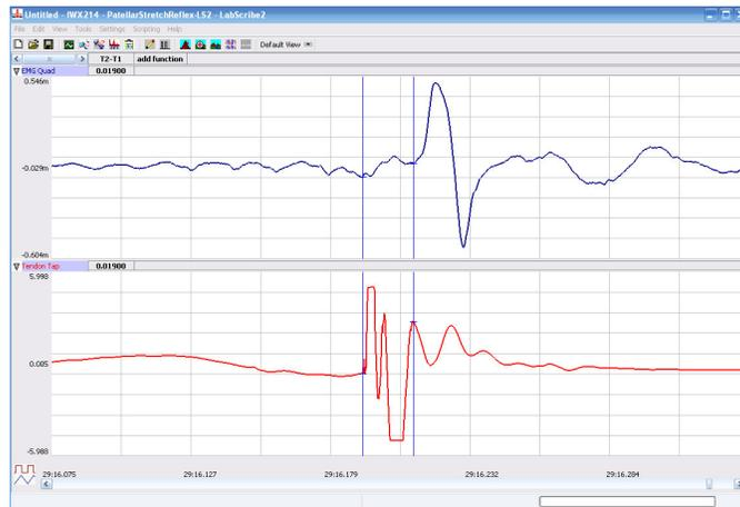
Figure NP-2-L3: An Achilles tendon reflex response and patellar hammer signal displayed on the Analysis window. The cursors are in position to measure the reflex conduction time
