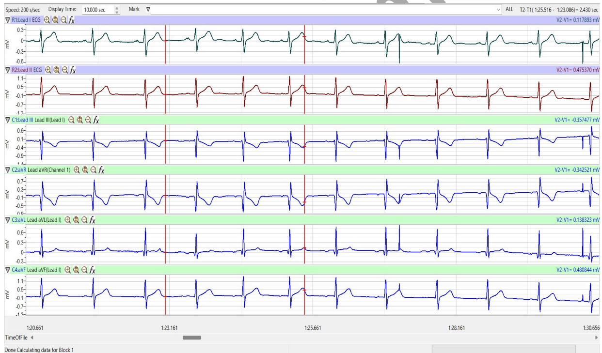
Figure HH-4-L1: Six lead ECG generated by recording Leads I and II on Channels 1 and 2, respectively. The remaining limb leads are derived by computed functions.
