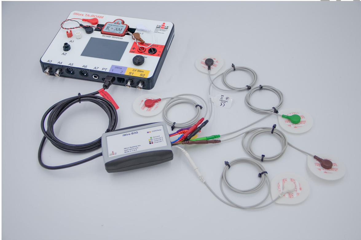
Figure HH-4-S1: The iWire-B3G ECG cable connected to an IXTA.
