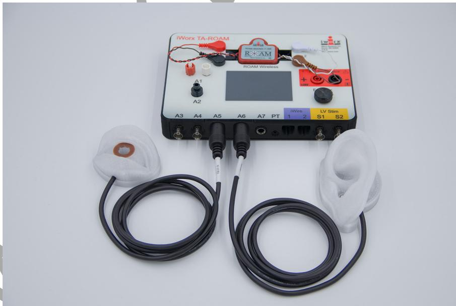
Figure HN-14-S2: The IXTA with the NMD-Eye and Ear plugged into channels 5 and 6 respectively.
