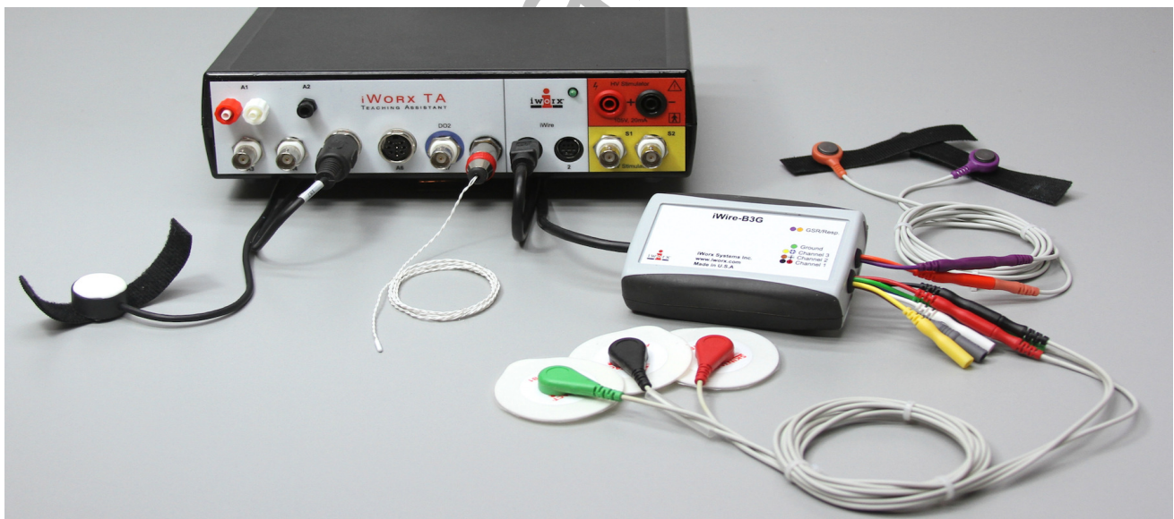
Figure HP-8-S3: The equipment needed to record the information for the Rubber Hand Illusion lab: EMG, GSR, pulse and temperature.
