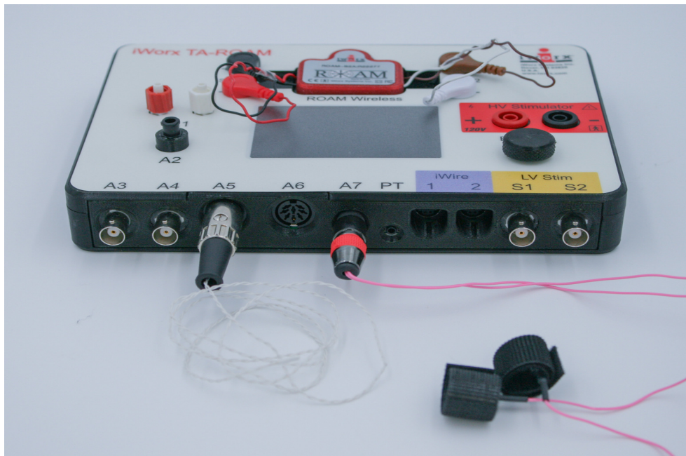
Figure HP-8-S3: The equipment needed to record the information for the Rubber Hand Illusion lab: GSR and temperature. Pulse will be plugged into the PT port.
