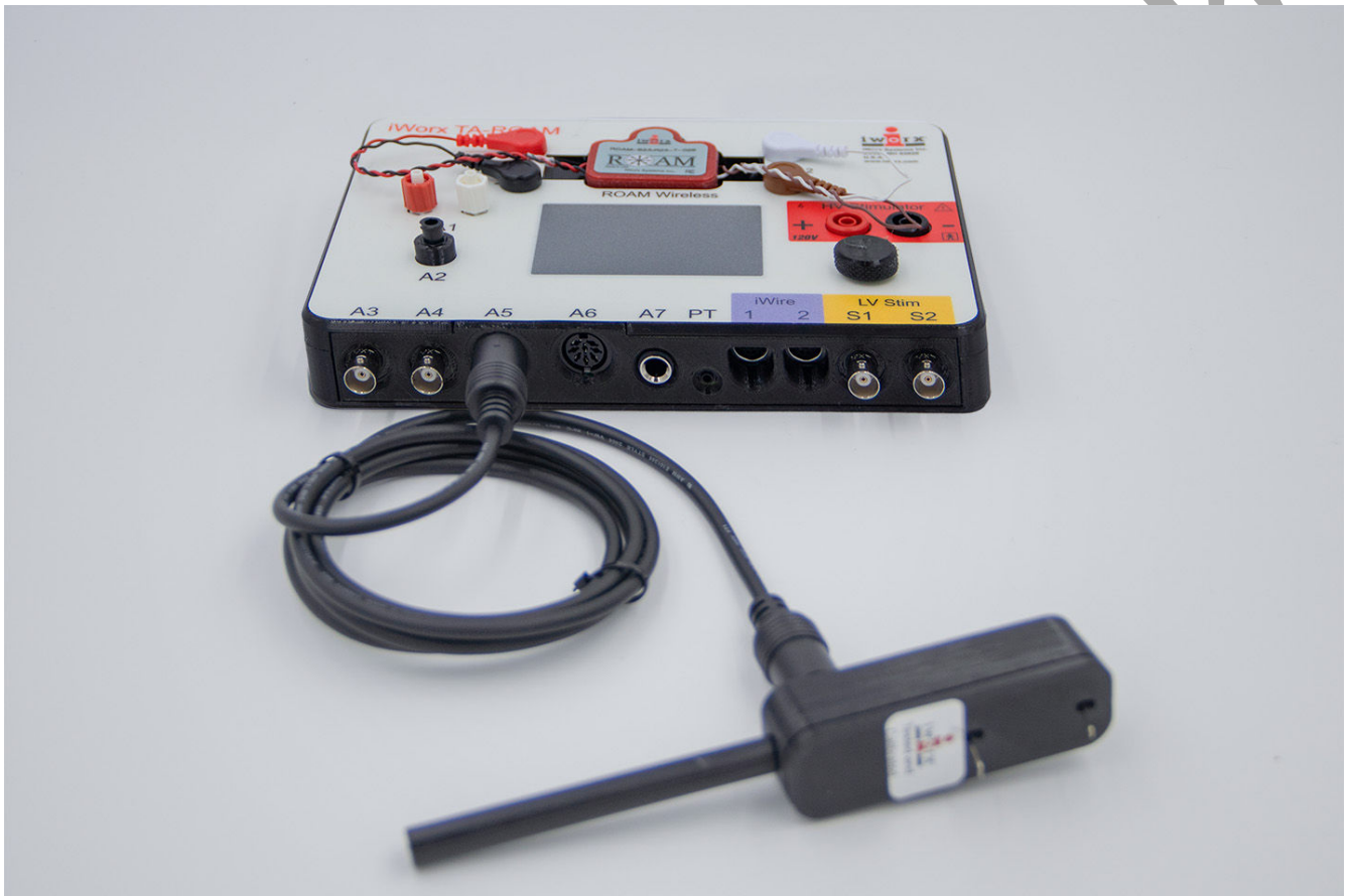
Figure AM-4-S4: The FT-302 dual-range force transducer connected to an IXTA.
