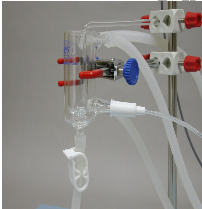
Figure AM-4-S6: 25 ml tissue bath in position for recording tissue tension.
