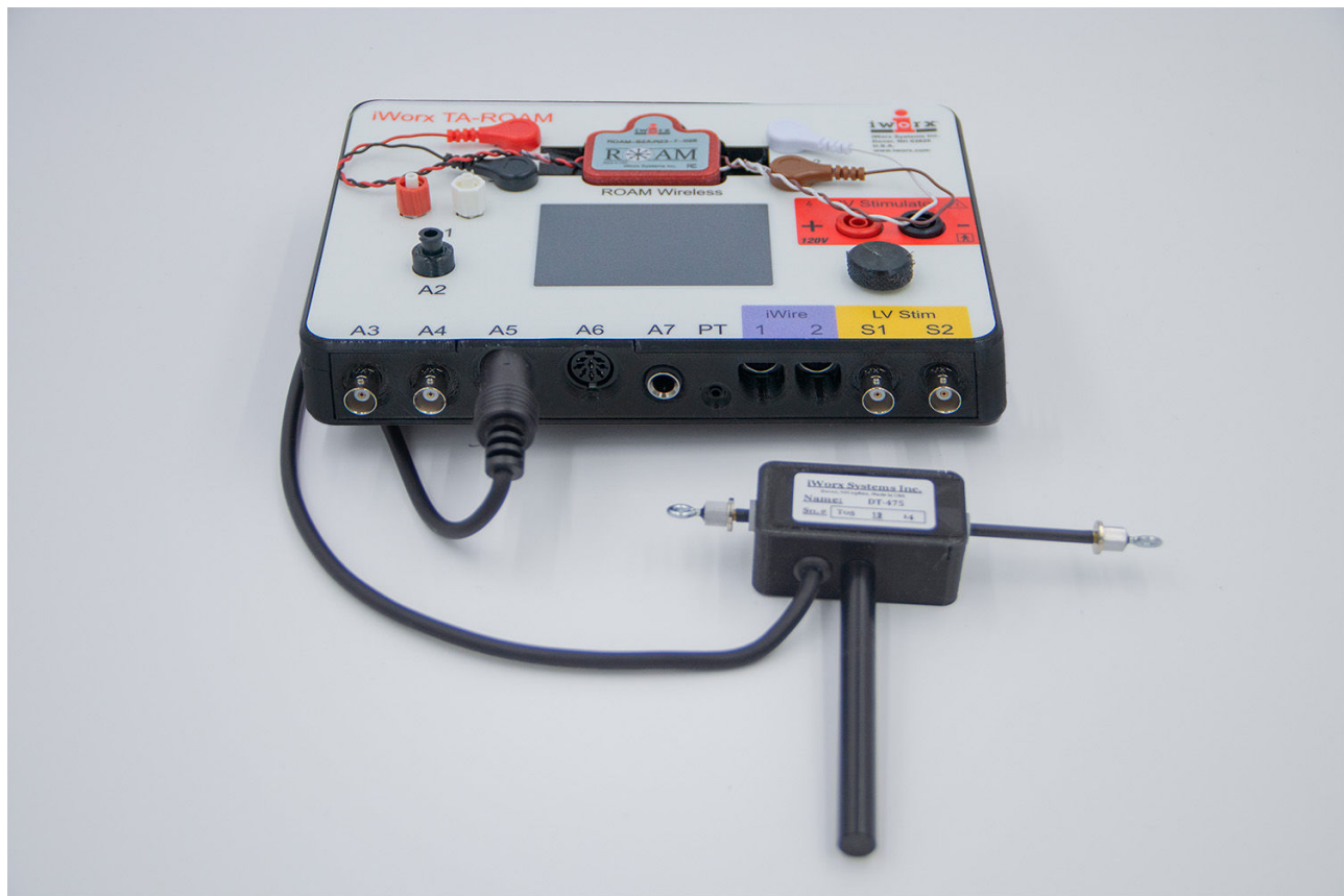
Figure AM-4-S2: The DT-475 displacement transducer connected to an IXTA.
