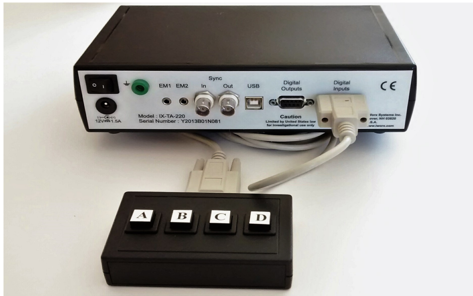
Figure HN-10-S2: The IX-TA with the RPD-400 event marker. The pulse sensor gets plugged into the front of the IX-TA to channel A-5.
