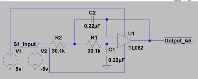
The Filter is a Sallen Key 2-pole low pass filter. Its job is to remove 60Hz electrical noise picked up from fluorescent lights, computers and AC power lines.
