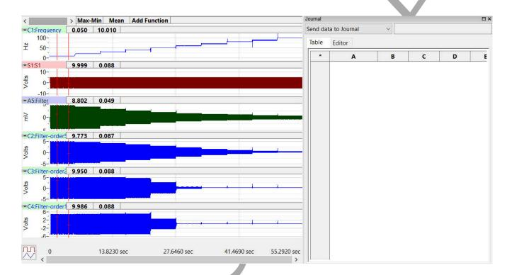
As you can see in the image above, the first graph show the input frequency. Place the 2 cursors on the flat portion so that you can see that the Mean frequency in the first graph is 10 Hz. The Max-Min of the rest of the channels shows the amplitude of the filter, which is about 10V.
