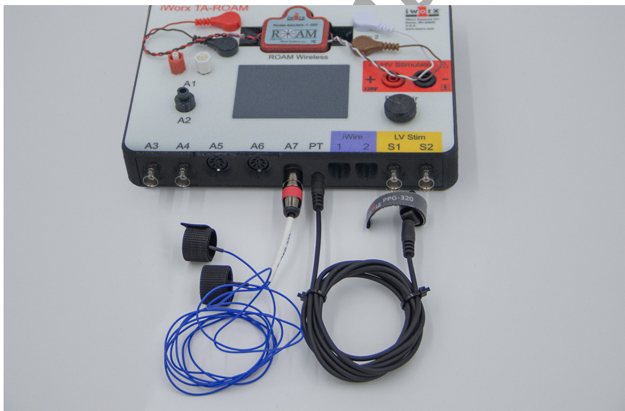
Figure HP-24-S2 The pulse sensor and GSR electrodes. Temperature will be plugged into A5.
