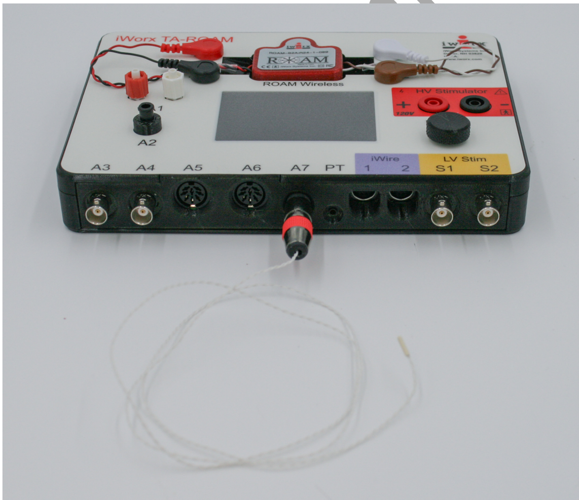
Figure BI-8-S1: The temperature sensor plugged into A7 on the front of the IX-TA
