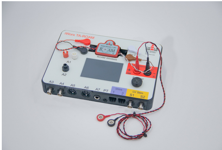
Figure HN-7-S3: The front panel of the IXTA with the stimulating electrodes connected correctly.
