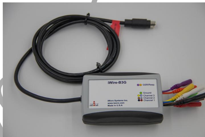
Figure AN-5-S1: The iWire-B3G recording cable.
