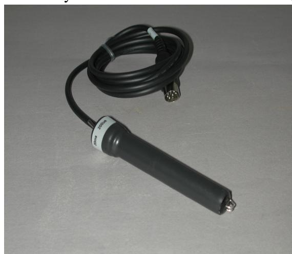
*Figure HK-2-S1: The CM-100 conductivity meter.*
