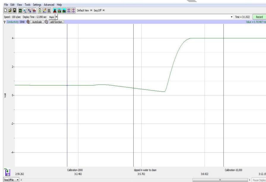
*Figure HK-2-S3: Conductivity calibration data recorded showing the positions of the cursors for changing the recorded voltage to conductivity in uS.*
