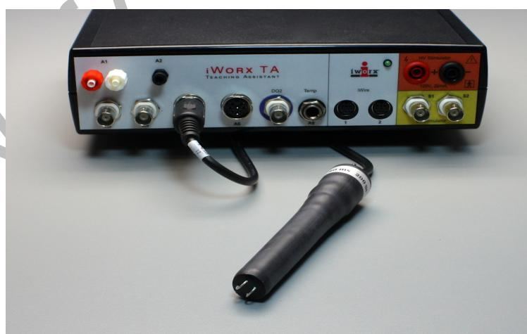
*Figure HK-2-S2: The CM-100 conductivity meter connected to the IXTA.*
