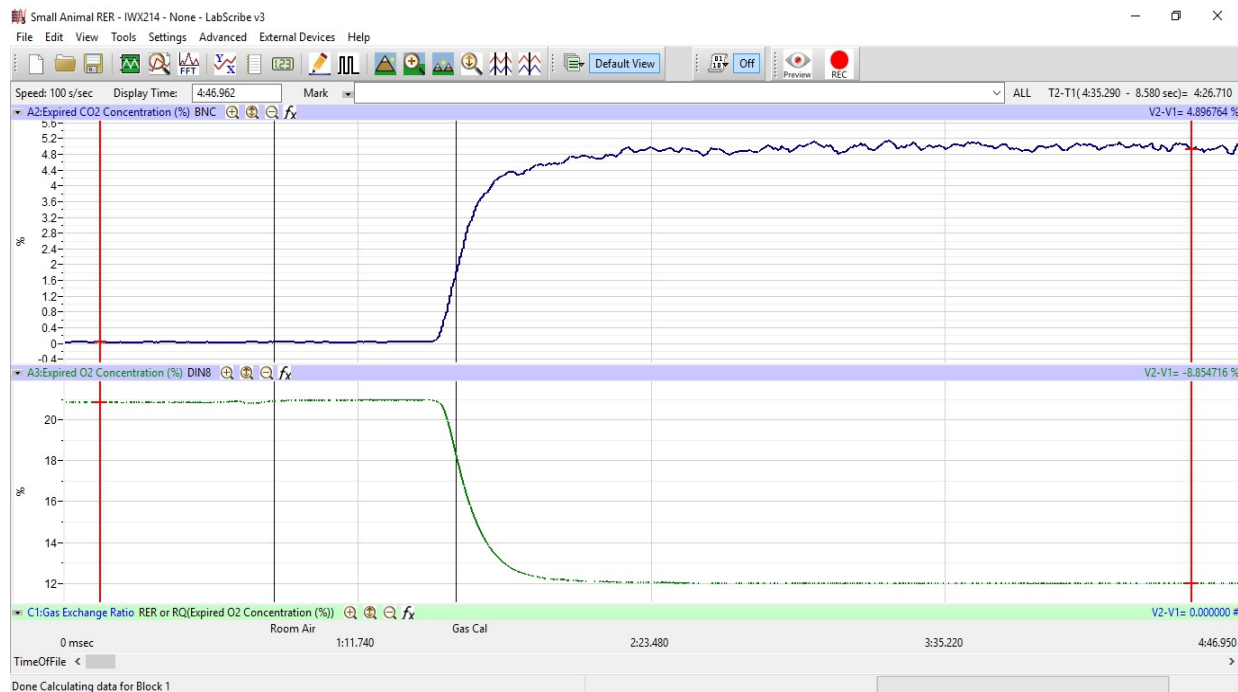
Figure AMe-3: The voltage outputs of the two sensors in the gas analyzer, carbon dioxide on the top and oxygen on the bottom. Other recording windows have been minimized to show detail.
